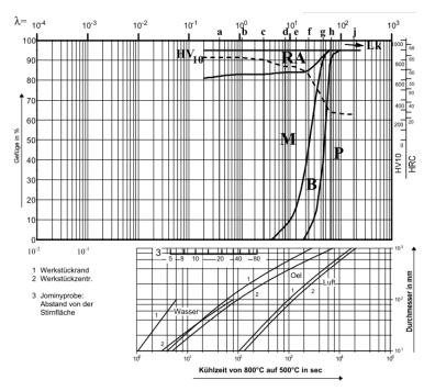
HV10... Vickers Hardness Lk... Ledeburite carbide RA... Residual austenite M... Martensite B... Bainite P... Perlite
